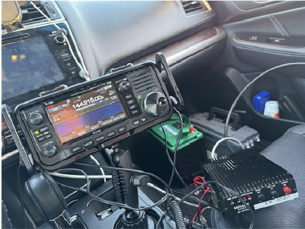
Icom 705 with small Mirage AMP running 70 watts with a 5 watt drive from the IF Rig
